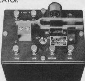
The 400-cycle TYPE 213-B Audio Oscillator whose waveform characteristics are shown on the opposite page
